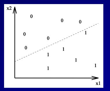
A linear threshold unit always produces a linear decision boundary. A set of points that can be separated by a linear decision boundary is said to be <u>linearly separable</u>.
