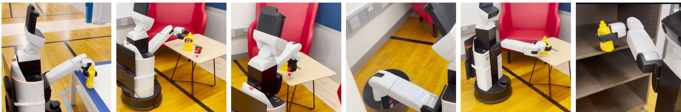
(a) grasp bottle (b) free gripper (c) grasp soup can (d) place soup can (e) re-grasp bottle (f) place bottle
