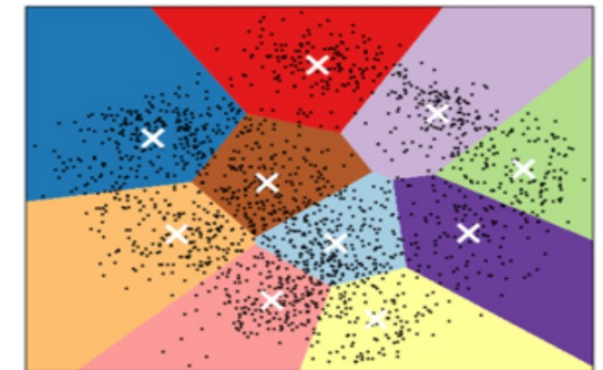
K-means clustering on the digits dataset (PCA-reduced data) Centroids are marked with white cross
