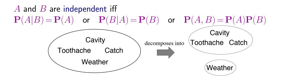
$$\begin{split} \mathbf{P}(Toothache, Catch, Cavity, Weather) \\ &= \mathbf{P}(Toothache, Catch, Cavity) \mathbf{P}(Weather) \end{split}$$
