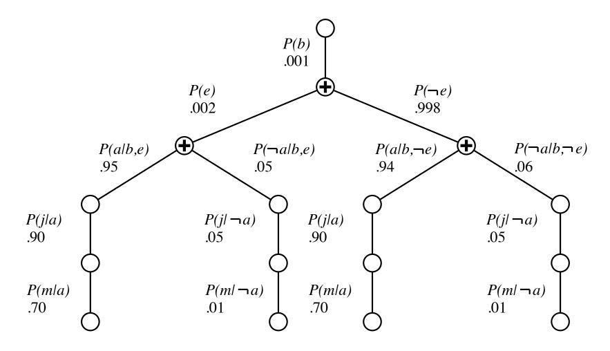
Enumeration is inefficient: repeated computation e.g., computes P(j|a)P(m|a) for each value of e Variable elimination: carry out summations right-to-left, storing intermediate results (factors) to avoid recomputation
