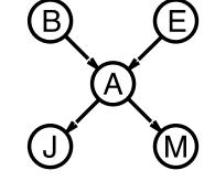
Rewrite full joint entries using product of CPT entries:  $\mathbf{P}(B|j,m) = \alpha \sum_{e} \sum_{a} \mathbf{P}(B)P(e)\mathbf{P}(a|B,e)P(j|a)P(m|a) = \alpha \mathbf{P}(B) \sum_{e} P(e) \sum_{a} \mathbf{P}(a|B,e)P(j|a)P(m|a)$
