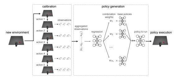
Figure 1: Illustration of policy self-evolution of POSEC using calibration actions. In a new environment, the agent executes the calibration actions to collect observations about the environment, predicts the combination weights of base polices, and obtains the final policy to run in the environment.
